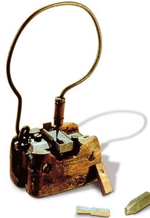
Hand casting instrument for casting lead type
